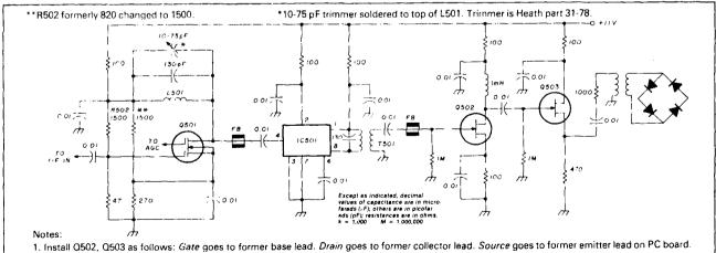
fig. 3. Partial schematic of the SB-104A i-f/audio board F showing modifications to improve strong-signal-handling capability.
